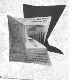
The Dreispitz is sundial and compass in one. We can determine the time and direction on the loop. This compass works well. It works with a north compass needle. The north compass needle has a fixed offset from the legal time. The legal time is against the legal longitude. The longitude difference is the angle between the indicated longitude and the longitude of observation. The angle is multiplied by 4 to yield the minutes that have to be added to the time shown by the Dreispitz.
