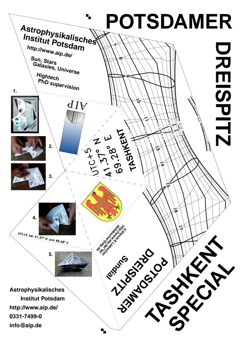
The *Dreispitz* is sundial and compass in one. We can determine the time and the north direction as well. This compass function, however, depends sensitively on the geographic latitude. It works well only for places with a geographic latitude like that indicated with an error of less than half a degree. When you know the north, the clock works well for latitudes that differ less than 8 degrees from the indicated one.
